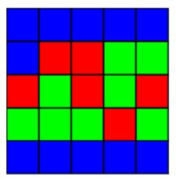
As you can see, longer stretches of a solid color make the file more compressible (lines 1 and 5 are the most compressed) and speckled images cannot compress (line 3 is not compressed at all). When the color changes with each pixel in a row, there is no shorter way to convey the information. So images with large blocks of the same colour compress very well. As data is not lost when the image is compressed the file format is lossless.
