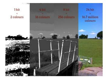
representing the maximum brightness of that colour). So to represent bright yellow the values 255, 255,0 can be used to represent the brightness of red, green and blue.
