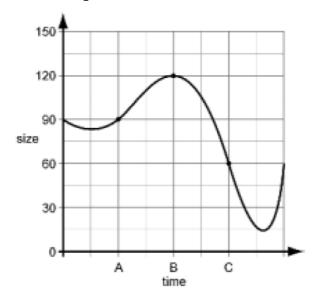
At point A on the graph, the size of the sound wave is 90. This is stored digitally using the binary value of 0101 1010 (or 5A in Hex). Complete the table below to show how points B and C are stored:
