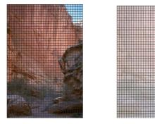
The image is split up into regions using a grid Each block in the grid is dealt with on its own.
