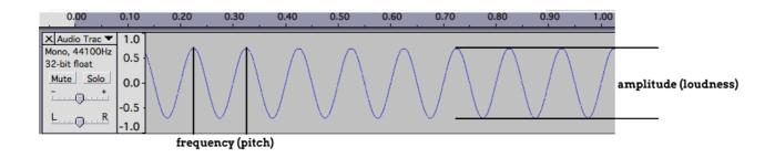
The distance between each peak is known as the frequency and is measured in hertz. The height of the wave (amplitude) corresponds to the loudness.
