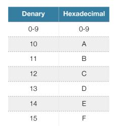
So if we want to display the number 12 as a hexadecimal number we would write C. We would write 20 in hexadecimal as 14 and we would write 31 in hexadecimal as 1F (one 16 and 15 units).
